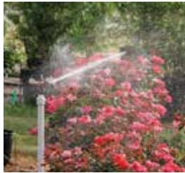
The 20 series WedgeDrive sprinkler alternately deflects flows in front and behind the splasharm as the wedge diffuser reacts to an incoming water stream. Its square orifice nozzle and rapid 360° rotation speed at low pressures delivers uniform distribution near and away from the sprinkler.
