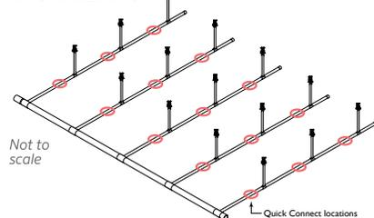
Senninger's Quick Connect Couplings make it easy to disassemble the system in manageable sections.
