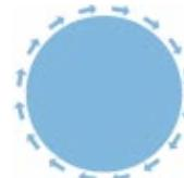
Ordinary rotating sprinklers have stationary legs that block water and create leg shadows. The Smooth Drive's walking diffuser eliminates bracket leg shadows resulting in unobstructed, uniform distribution.
