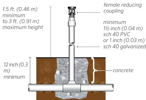
NOTE: Care must be taken to stabilize the riser. For other installation details, contact our factory.
